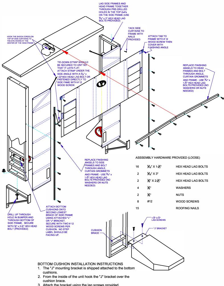
Attach the bracket using the lag screws provided.
